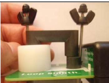
4. While continuing to push on bolt heads as in step 1, use fingers from other hand to tilt right bolt (see photo above) and then disengage this bolt from right slot of upper ferrite. Lift upper ferrite and gently swing it away from tilted bolt while keeping ferrite left side captured in white nylon bushing.
